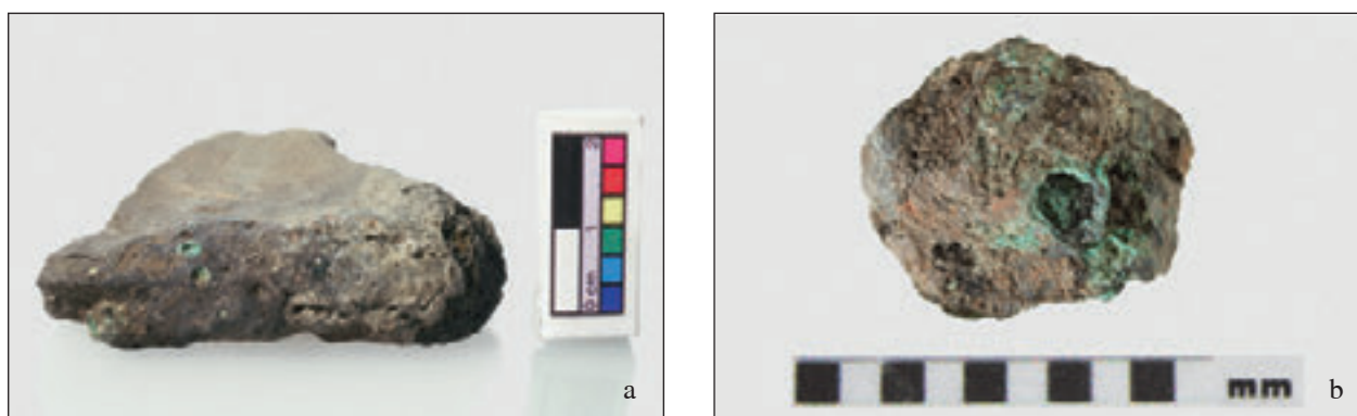
Fig. 2. a) A slagged ceramic sherd from Belovode (31b); b) An individual slag sample from Belovode (134)
