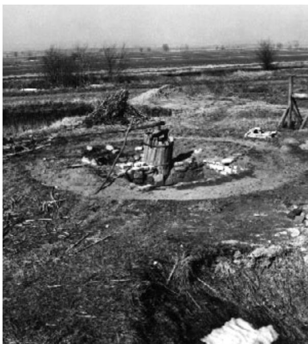
*Fig. 30. Device for mixing and grinding clay (driven by draft animals) on a private estate in the Požarevac area (east Serbia). Right: a well (photo M. Jeremić)*
