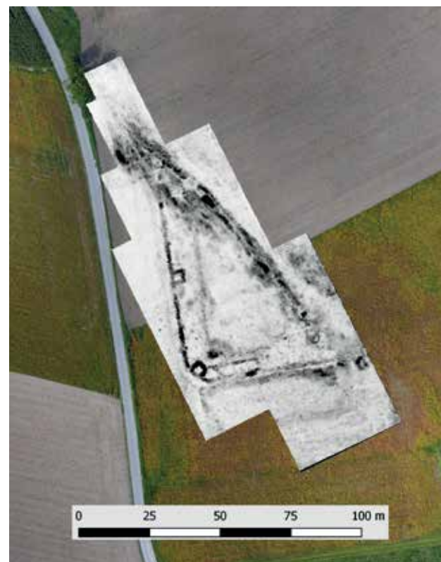
Fig. 8 - Radargram (summed depth slices from -0.50 to -0.70 m) of the fort area in Stein (ArchaeoPublica – G. Grabherr/B. Kainrath)
