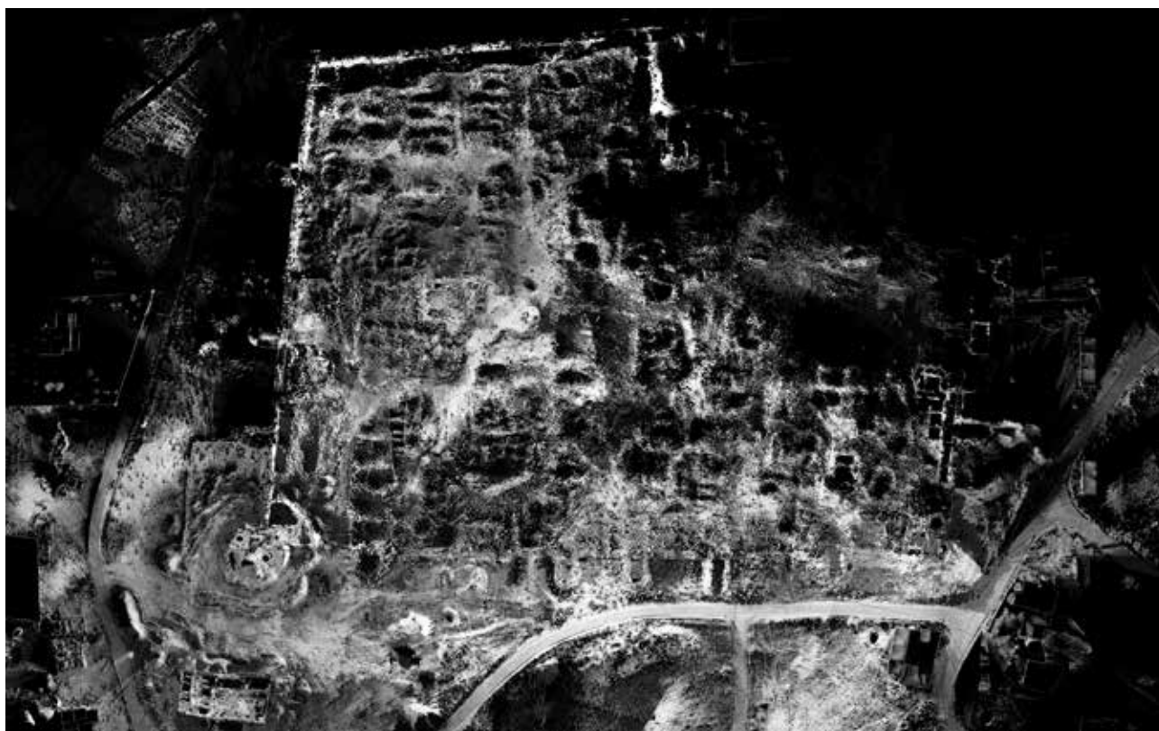
Fig. 7 - 3D reconstruction of the southern curtain wall of the Udhrūh castra and environs, made with Leica P30 scanstation. Made by Maarten Sepers.
