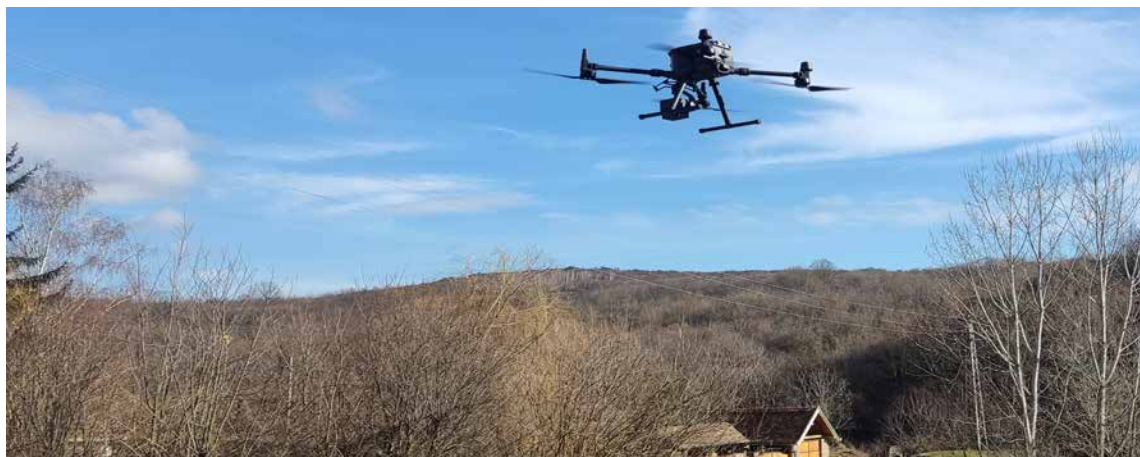
Figure 2. DJI Matrice 350 RTK with Zenmuse L2 camera. (Photo by P. Milojević).
