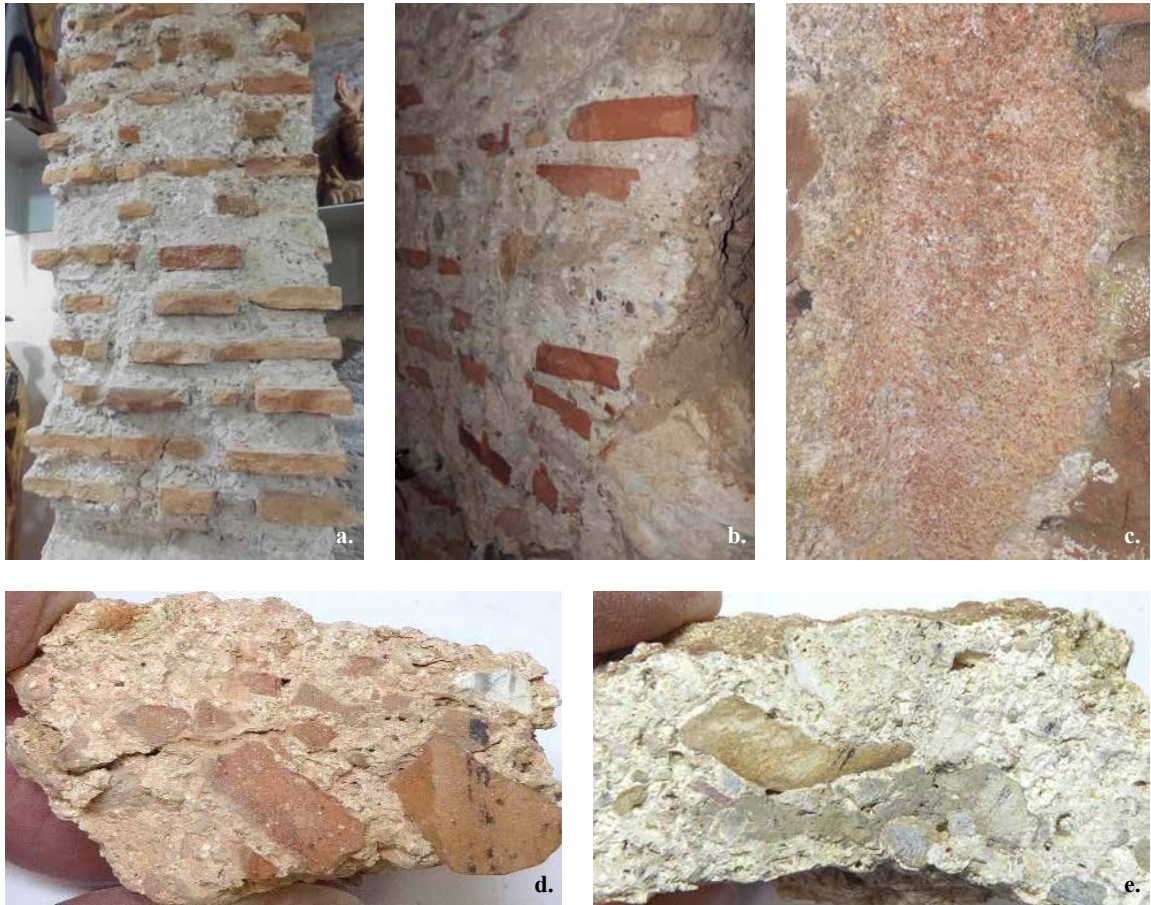
Figure 7. Most probably dry slaked and sieved or screened mortars: a. building and b. first coat plaster of Roman masonry preserved beneath the Gothic cathedral in Valencia (photos taken by Nigel Copsey); c. Cocciopesto plaster mortar, Viminacium Bath House, sawn surface (photo taken by Bill Revie); d. Cocciopesto plaster mortar, Ravenglass Roman Bath House (photo taken by Nigel Copsey); e. Bricklaying mortar, Viminacium, sawn surface (photo taken by Bille Revie).
