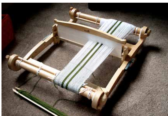
Figure 15. A modern home rigid heddle loom (photo taken from: https://www.flickr.com/photos/origamichan/3639603898/ ). Photograph copyright © Tokyotogo – CC BY-NC-ND 2.0 (accessed on December 12 th , 2024).
