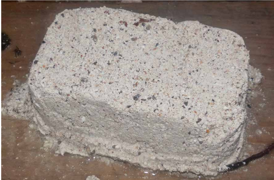
Figure 18. Sample reproduction of typical 18 th C bricklaying mortar, 4 lime: 1 sharp sand, dry slaked and hot mixed. Made by the author (photo taken by Nigel Copsey).
