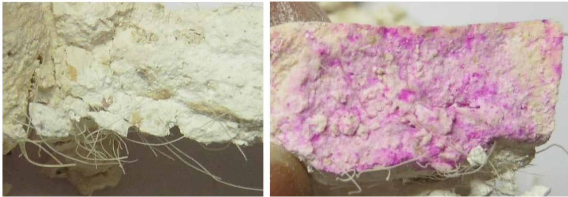
Figure 22. Carbonation of dry slaked lime and hair mortar after 10 months in situ (photos taken by Bille Revie).
